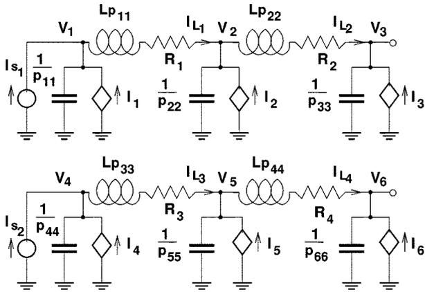
Fig. 1. PEEC circuit: two wires, two cells in each wire.
