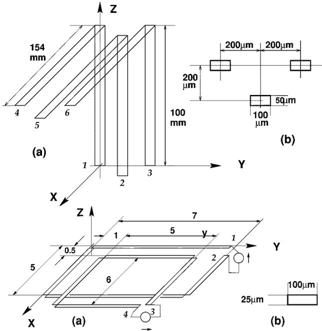
Fig. 2. Top: (a) three wires with bend and (b) cross-section. Bottom: (a) two loops and (b) cross-section 1w.
