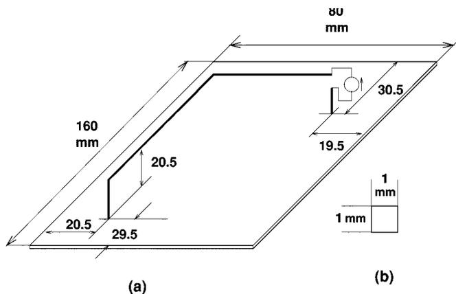
Fig. 6. Loop over ground plane.
