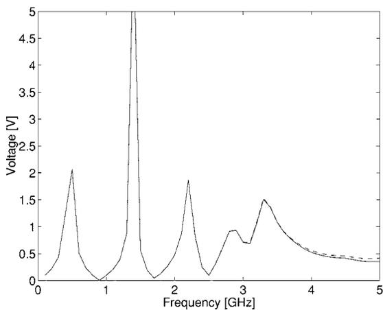
Fig. 7. Magnitude of output voltage for loop over plane. Frequency-domain analysis (—). MOR computation (---).
